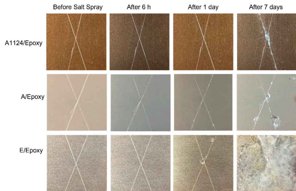
Figure 16. Macroscopic images of the x-cut samples after salt spray test.
